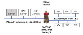
Segments 2 existing BACnet MS/TP networks from a new BACnet/SC network. BACnet Firewall filtering.
