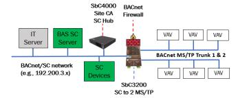
Segments 2 existing BACnet MS/TP and 1 BACnet/IP network from a new BACnet/SC network. BACnet Firewall filtering.
