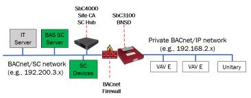
3. Creates a BACnet/IP private network when IT limits fixed IP addresses or device access.
