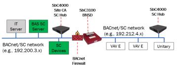
2. Segments existing BACnet/IP network to enable communication with BACnet/SC Networks.
